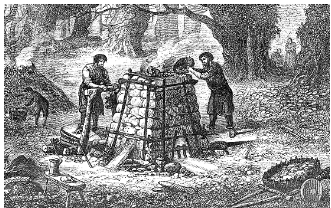
Quaint drawing of a bloomery – note operation of bellows
